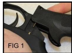
1. With rifle turned upside down, remove original handgrip taking care not to lose the safety selector spring and detent. Remove spring from grip and leave detent in the lower receiver.
