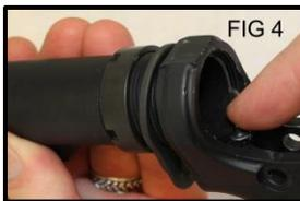
5. Remove original receiver endplate and replace with ergonomic receiver endplate. Reassemble buffer tube, reversing the order of disassembly. Retighten castle nut to apprx. 40 inch LB. **DO NOT USE THREADLOCKER.**
