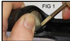
2. Using a stock wrench or multi tool, loosen and unscrew castle nut enough for original receiver endplate to slide back about 1/4". (FIG 2)
