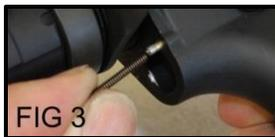
4. Rotate buffer tube another 1/4 turn keeping finger over retaining pin and spring to prevent them from flying out (FIG 4). Set aside and unscrew buffer tube.
